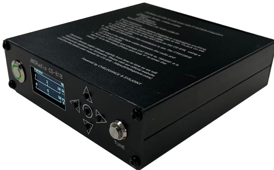
When working with Yaesu FT-817/818, CS-818 interfaces to the CAT port (ACC) on the back of FT-817/818 radio with the provided cable. The tuning process is very simple: Press the tune button on CS-818 and it will automatically switch the radio to PKT mode, transmit a carrier, tune the antenna, then restore the radio to the previous mode. CS-818 will also function as a general purpose antenna tuner with other QRP radios. Just transmit a carrier and press the tune button on the tuner.
